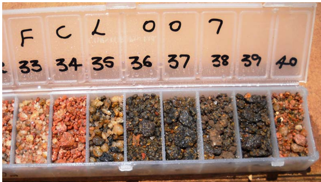
Figure 3.8: Oxidised Mineralisation (34 – 39m in FCL007: 5m @ 37.0% Fe)
