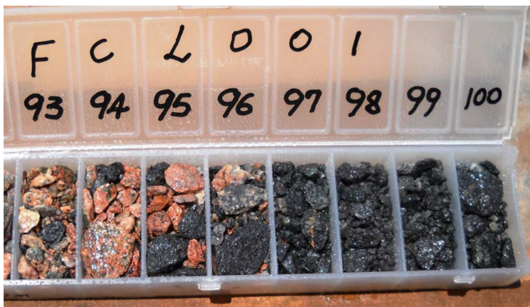
Figure 3.9: Fresh Mineralisation (94 – 100m in FCL001: 6m @ 30.1% Fe)
